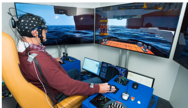
Figure 3: Measuring human performance in a MARIN simulator
